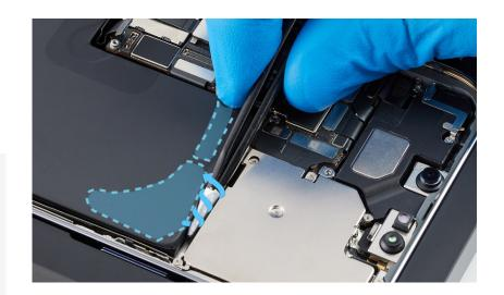
11. Repeat steps 9 and 10 to remove the remaining battery adhesive strip from the top of the battery. If you remove the entire strip, continue to step 12.
