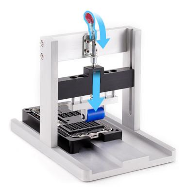
12. Slide the repair tray back and forth through the battery press three times to adhere the battery to the enclosure.
