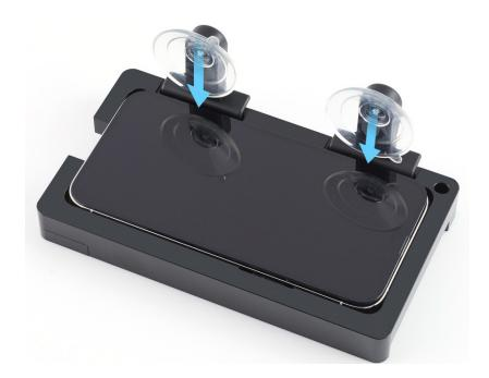
20. Tilt up the display toward the suction cups. Press the top and bottom edges of the display to secure it to the suction cups.
