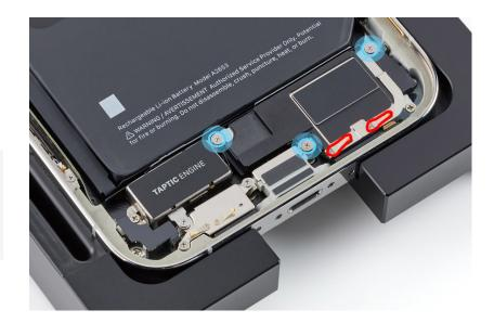
4. Use the blue torque driver and JCIS bit to install one new crosshead screw into the bottom speaker.
