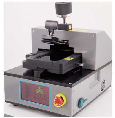
7. Turn the knob on the fixture clockwise to lower the suction cup as close to the iPhone as possible without touching the iPhone.
