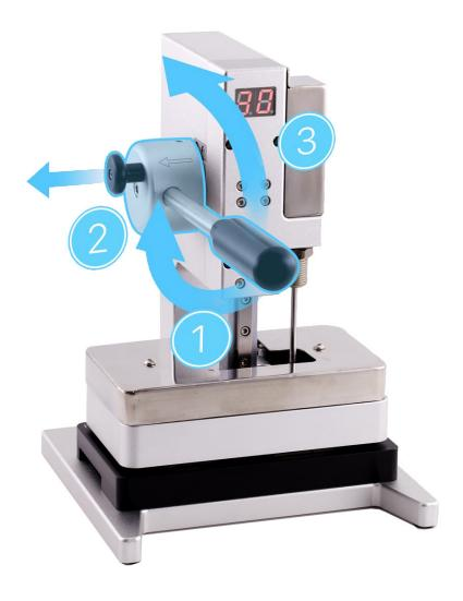
29. Remove the repair tray from the display press.
