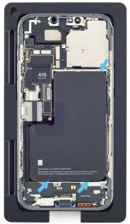
14. Slightly lift the battery with the black stick just enough to grasp underneath the battery.
