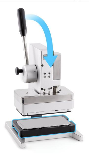
9. Wait until the timer on the display press beeps. Pull down the lever (1) and pull out the release knob (2). Then lift the lever (3).
