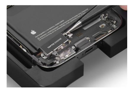
3. Press the end of the Taptic Engine flex cable to the connector.
