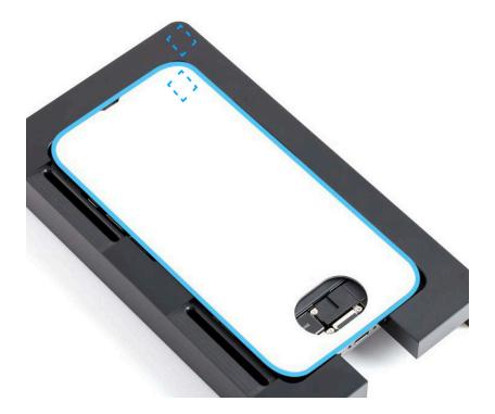
8. Position the repair tray with the iPhone in the display press. Pull down the lever until the display press locks.
