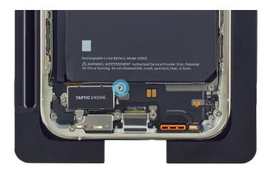
3. Use a torque driver and the JCIS bit to remove the two crosshead screws from the Taptic Engine. Set aside the screws.
