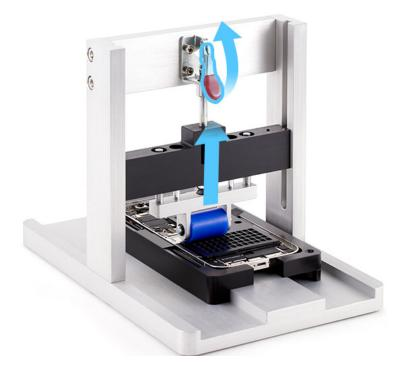
10. Position the repair tray and enclosure onto the battery press with the right slot over the pin.
