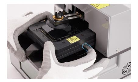
14. Hold both sides of the pocket and slide it straight out of the fixture.
