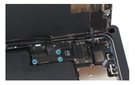
18. Use ESD-safe tweezers to slide the tab of the upper cowling behind the ambient light sensor flex cable. Then lower the cowling over the end of the flex cable.
