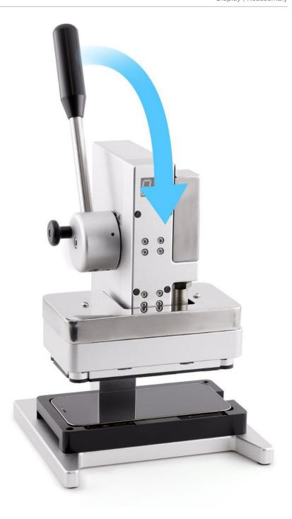
28. Wait until the timer on the display press beeps. Pull down the lever (1) and pull out the release knob (2). Then lift the lever (3).
