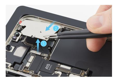
5. Use ESD-safe tweezers to lift the ends of the two camera flex cables off the connectors.
