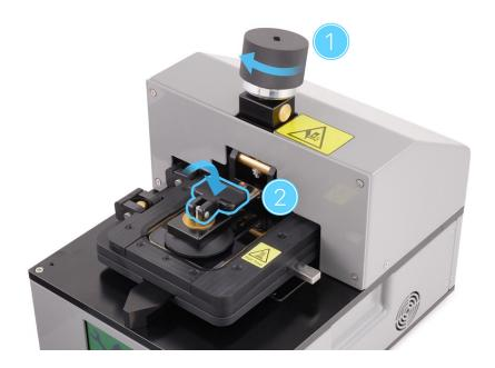
Slowly turn the knob on the fixture counterclockwise until the display begins to separate from the enclosure.
