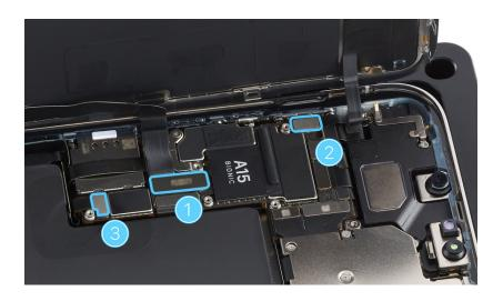
Use ESD-safe tweezers to position the lower cowling over the ends of the display and battery flex cables.
