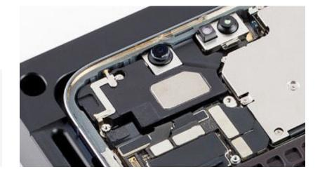
4. Align the replacement display adhesive over the enclosure with the grounding foam on top. Ensure that the top holes of the adhesive align over the TrueDepth camera assembly.
