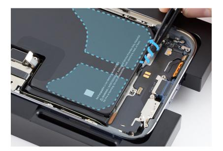
5. Pull the tweezers toward the bottom of the iPhone and continue to twist the adhesive strip until you've removed the entire strip.
