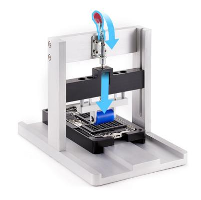
8. Slide the repair tray back and forth through the battery press three times to adhere the battery to the enclosure.
