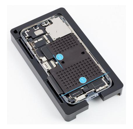
6. The center of the repair tray has two slots. Position the repair tray and enclosure onto the battery press with the left slot over the pin as shown.
