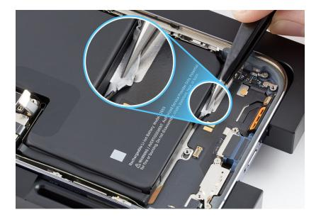
4. Keep the tweezers close and parallel to the battery and twist until you see white adhesive strip on the tweezers.
