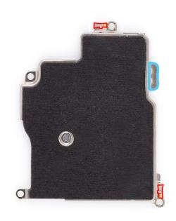
Hold the cowling with ESD-safe tweezers and slide the cowling tab into the slot. Then lower the cowling onto the cameras.
