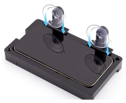
20. Tilt up the display toward the suction cups. Press the top and bottom edges of the display to secure it to the suction cups.
