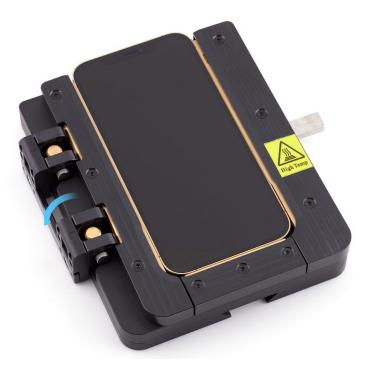
5. Put on the heat-resistant gloves. Align the cutout on the bottom of the pocket with the rail on the fixture. Slide the pocket with the iPhone onto the rail on the fixture.
