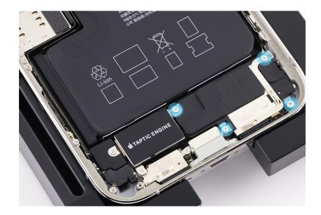
4. Use ESD-safe tweezers to remove the battery shim from the enclosure. Discard the shim.
