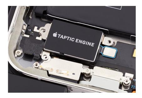
3. Use the gray torque driver and super screw bit to install two new super screws into the Taptic Engine.
