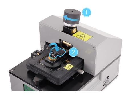
10. Slowly turn the knob on the fixture counterclockwise until the display begins to separate from the enclosure.
