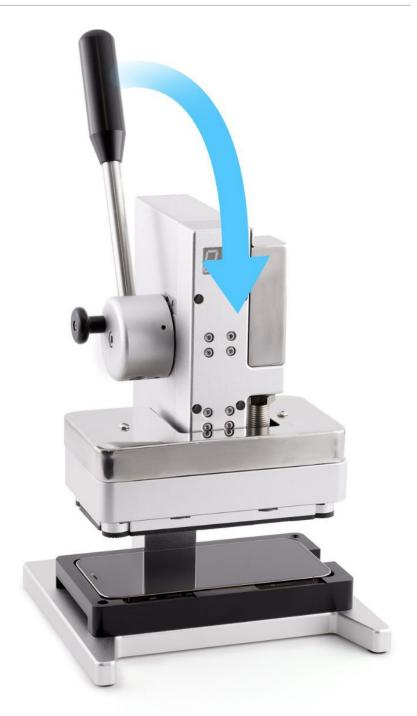
25. Position the repair tray with the iPhone in the display press. Pull down the lever until the display press locks.
