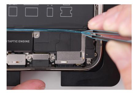
Run the flat end of the black stick between the replacement battery shim and the bottom edge of the battery to adhere the shim to the Taptic Engine and speaker.
