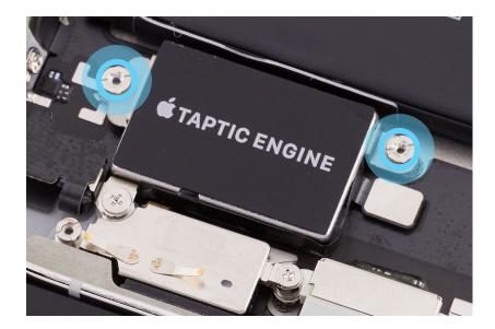
5. Use a torque driver and the JCIS bit to remove one crosshead screw from the Taptic Engine. Set aside the screw.
