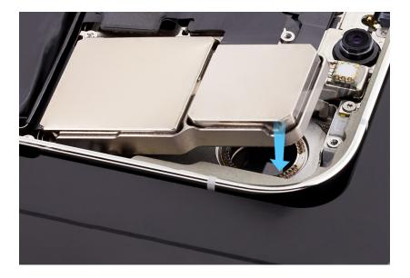
4. Press the end of the bottom camera flex cable to the connector.
