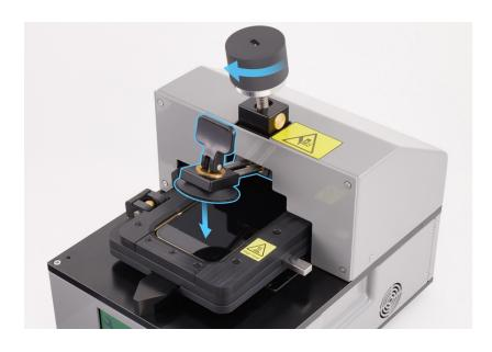
Grasp the handle and slide the suction cup straight out until the edge of the suction cup aligns with the bottom edge of the display.
