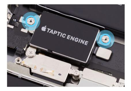
4. Use the green torque driver and JCIS bit to install one new crosshead screw into the Taptic Engine.
