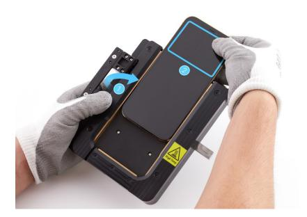
16. Place the iPhone into the repair tray with the display faceup and the Lightning connector facing the cutout. Remove the gloves.
