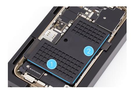
9. The center of the repair tray has two slots. Position the repair tray and enclosure onto the battery press with the left slot over the pin.
