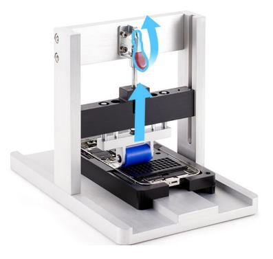
13. Position the repair tray and enclosure onto the battery press with the right slot over the pin.
