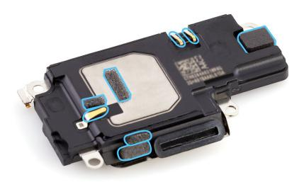
3. Rotate the repair tray. Align the port on the speaker with the hole in the enclosure. Then lower the speaker into position.
