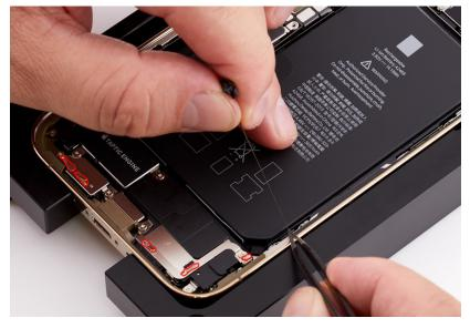
31. Use ethanol wipes or IPA wipes to clean any adhesive residue from the enclosure.
