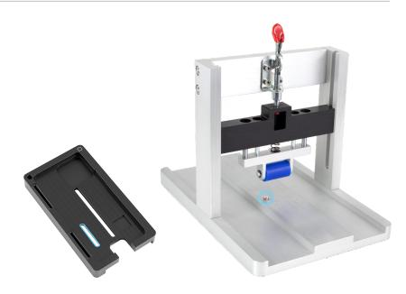
10. Flip down the red lever to lower the roller onto the battery.
