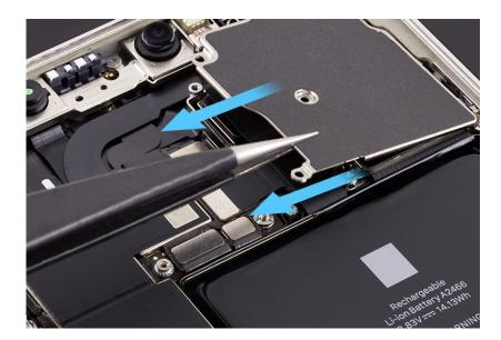
4. Use ESD-safe tweezers to lift the end of the top camera flex cable off the connector.
