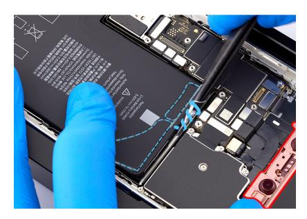
12. Repeat steps 10 and 11 to remove the remaining adhesive strip from the top of the battery. If you remove the entire strip, continue to step 13.
