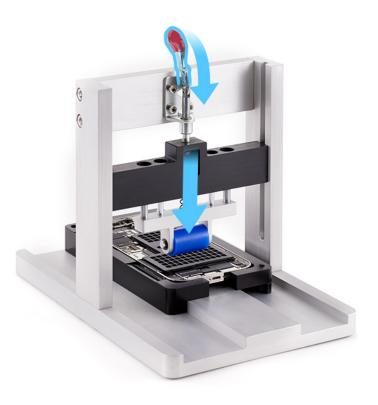
11. Slide the repair tray back and forth through the battery press three times to adhere the battery to the enclosure.
