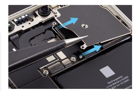
9. Hold the camera cowling in place with your finger. Use the green torque driver and Micro stix bit to install five new trilobe screws into the camera cowling in the order shown.
