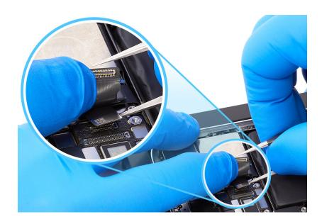
6. Gently hold the flex cables together and lift the cameras out of the enclosure.
