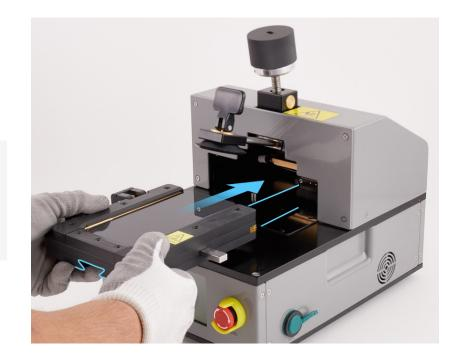
6. Slide the pocket into the fixture until you hear the pocket click into place.
