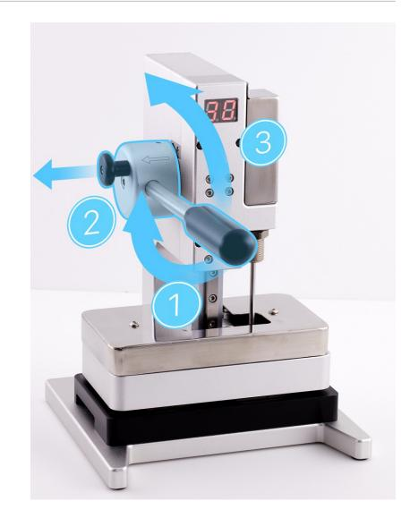
26. Wait until the timer on the display press beeps. Pull down the lever (1) and pull out the release knob (2). Then lift the lever (3).
