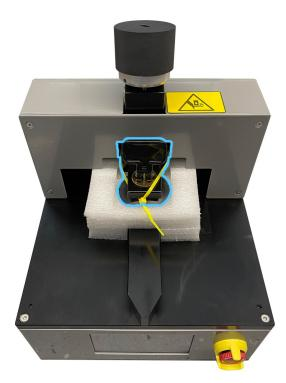
Turn the top knob on the fixture counterclockwise to raise the suction cup. Remove the packing Styrofoam.
