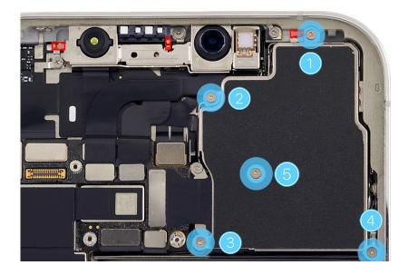
3. Use ESD-safe tweezers to tilt up the camera cowling from the left side. Then slide the cowling tab out of the slot on the right of the enclosure. Save the cowling for reassembly.
