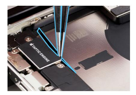
6. Use the flat end of the black stick to adhere the battery shim to the Taptic Engine and speaker.
