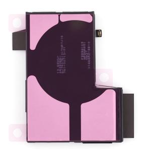
8. Hold the battery over the enclosure with the protective cover faceup. Align the bottom of the battery with the Taptic Engine (1) and the right edge with the enclosure (2). Then lower the battery into the enclosure.
