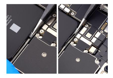
10. Hold down the iPhone. Use ESD-safe tweezers to grasp one battery adhesive tab. Twist the tweezers to wrap the adhesive strip around them.
