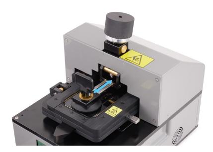
Turn the knob on the fixture clockwise to lower the suction cup onto the display (1). Then flip down the handle on the suction cup to secure the suction cup to the display (2).
