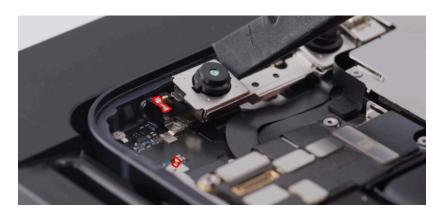
4. Align the replacement display adhesive over the enclosure with the top holes over the TrueDepth camera assembly and the bottom tab on the right.
