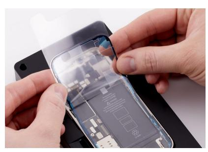
6. Place the display adhesive press plate on top of the enclosure with the icon in the top right corner as shown.
