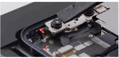
4. Align the replacement display adhesive over the enclosure with the top holes over the TrueDepth camera assembly and the bottom tab on the left.
