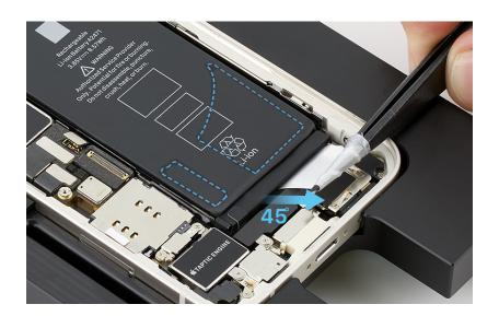
5. Use ESD-safe tweezers to grasp the bottom left battery adhesive tab and gently peel it away from the battery.
