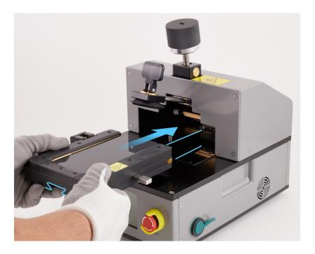
6. Slide the pocket into the fixture until you hear the pocket click into place.
