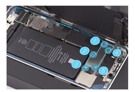
19. Peel the first strip from the middle release liner (1) counterclockwise, starting at the top right of the enclosure. Peel the second strip (2) clockwise, starting at the top right of the enclosure. Peel the third strip (3) clockwise, starting at the bottom left of the enclosure.
