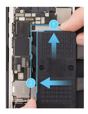
4. The center of the repair tray has a slot. Position the repair tray and enclosure onto the battery press with the slot over the pin.
