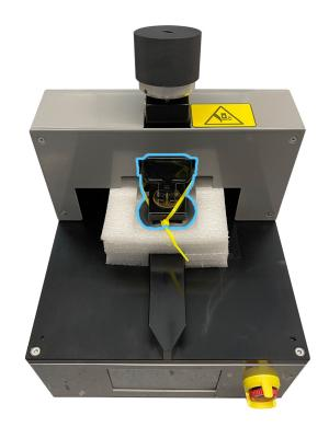
3. Turn the top knob on the fixture counterclockwise to raise the suction cup. Remove the packing Styrofoam.
