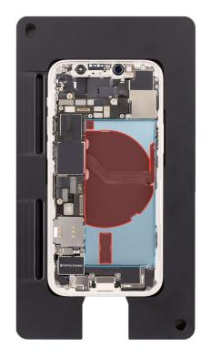
13. Insert the flat end of the black stick into one of the insertion points as shown. Ensure that the black stick is inserted into a point where the battery strip has been fully removed. Don't insert the black stick into a point where the battery tab or strip is broken.
