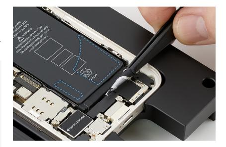
4. Pull the tweezers outward at a 45-degree angle and continue to twist the adhesive strip until you've removed the entire strip.
