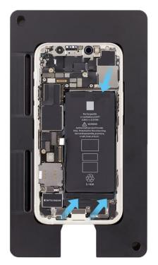
14. Slightly lift the battery with the black stick just enough to grasp underneath the battery.
