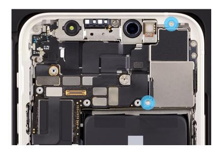
3. Use ESD-safe tweezers to tilt up the left side of the camera cowling as shown. Then slide the camera cowling out of the enclosure. Save the cowling for reassembly.
