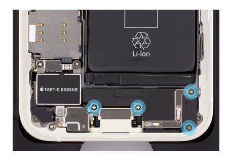
3. Use the black stick to tilt up the speaker. Then grasp the area outlined in blue and remove the speaker from the enclosure.
