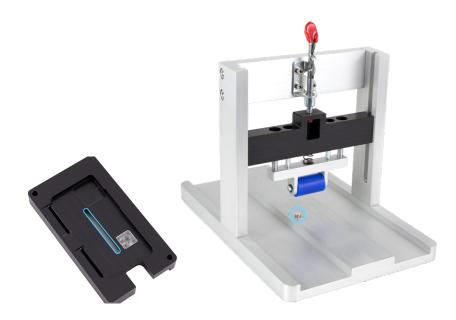
5. Flip down the red lever to lower the roller onto the battery.
