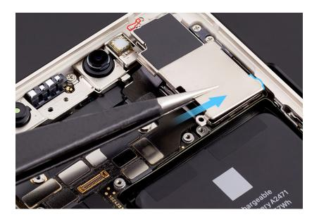
8. Use the gray torque driver and JCIS bit to install two new crosshead screws into the camera cowling.
