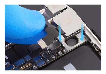
3. Press the end of the bottom camera flex cable to the connector.
