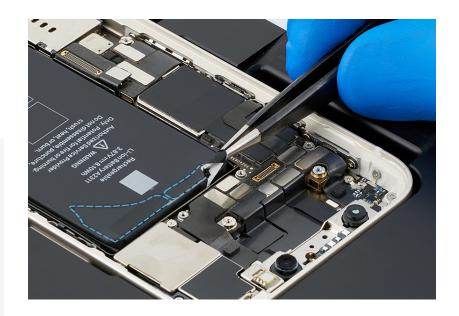
10. As the adhesive strip stretches, continue to slowly pull and twist the tweezers until you've removed the entire strip.
