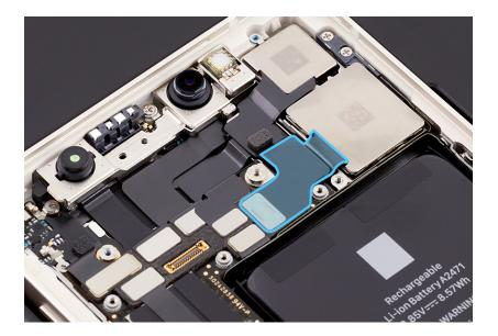
5. Lift the end of the bottom camera flex cable off the connector.
