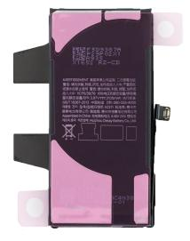
3. Hold the battery over the enclosure with the protective cover faceup. Align the top of the battery with the cameras (1) and the left edge with the logic board (2). Then lower the battery into the enclosure.
