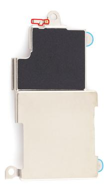
7. Hold the cowling with ESD-safe tweezers and slide the cowling tabs into the slots. Then lower the cowling onto the cameras.
