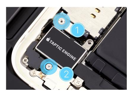
5. Position the Taptic Engine connector cowling over the end of the flex cable.
