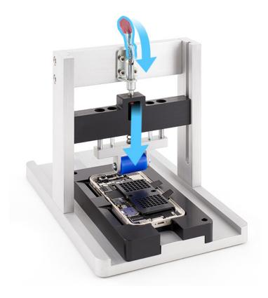
6. Slide the repair tray back and forth through the battery press three times to adhere the battery to the enclosure.
