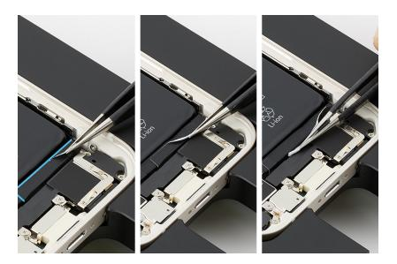
3. Hold down the iPhone. Use ESD-safe tweezers to grasp the battery adhesive tab. As the strip stretches, twist the tweezers to wrap the battery adhesive around them.
