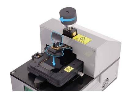
8. Grasp the handle and slide the suction cup straight out until the edge of the suction cup aligns with the bottom edge of the display.
