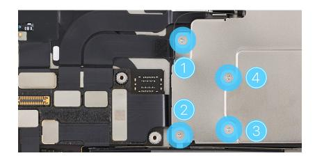
Use ESD-safe tweezers to remove the camera cowling. Save the cowling for reassembly.
