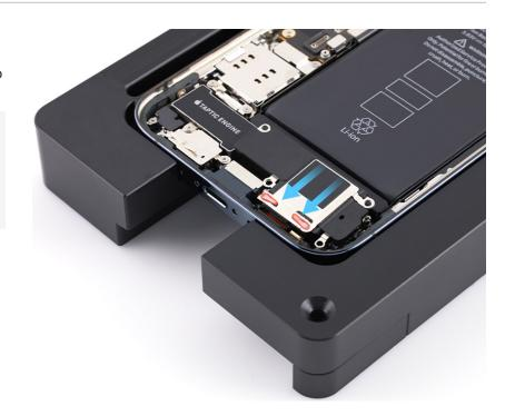
4. Use the green torque driver and JCIS bit to install four new crosshead screws into the speaker.
