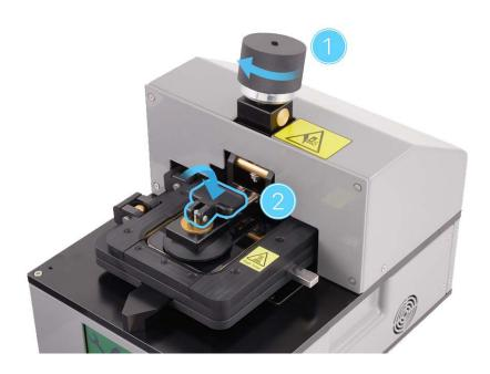
10. Slowly turn the knob on the fixture counterclockwise until the display begins to separate from the enclosure.
