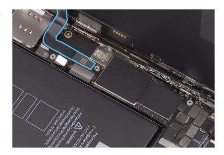
28. Use the black stick to lift the end of the Multi-Touch flex cable off the connector.
