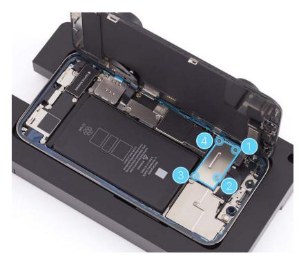
Peel the first strip of the middle release liner (1) counterclockwise, starting near the bottom of the enclosure. Peel the second strip (2) clockwise, starting near the bottom of the enclosure. Peel the third strip (3) counterclockwise, starting near the top of the enclosure.
