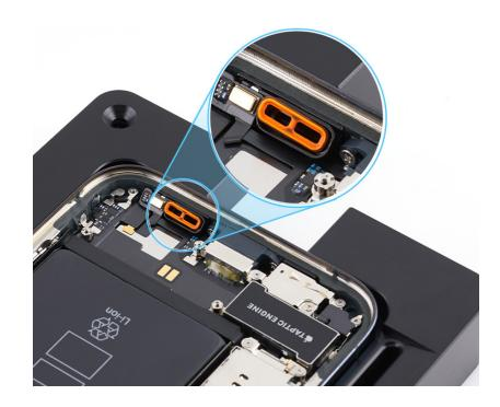
2. If the rubber gasket is out of position, use ESD-safe tweezers to reposition it.
