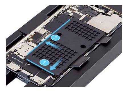
6. The center of the repair tray has two slots. Position the repair tray and enclosure onto the battery press with the left slot over the pin as shown.
