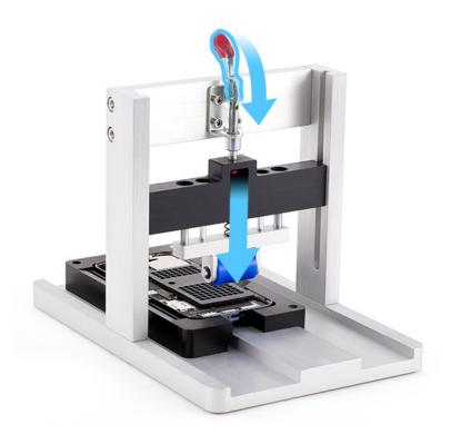
12. Slide the repair tray back and forth through the battery press three times to adhere the battery to the enclosure.
