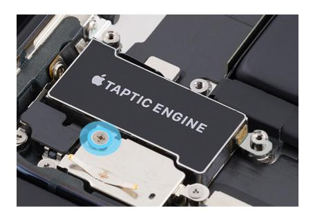
4. Use the gray torque driver and super screw bit to install two new super screws into the Taptic Engine.
