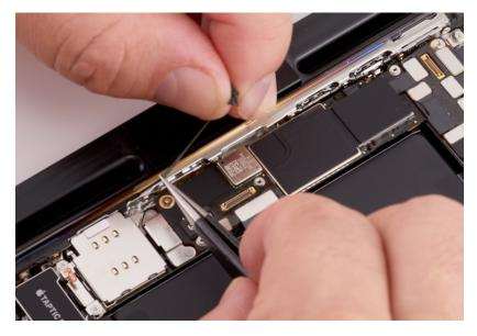
33. Use ethanol wipes or IPA wipes to clean any adhesive residue from the enclosure.
