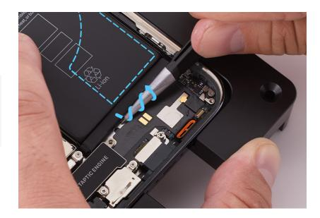
6. Pull the tweezers toward the bottom of the iPhone and continue to twist the adhesive strip until you've removed the entire strip.
