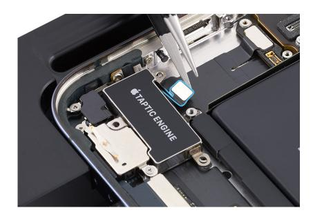
15. Use ESD-safe tweezers to remove the Taptic Engine.
