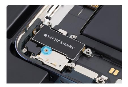
14. Use ESD-safe tweezers to lift the end of the Taptic Engine flex cable off the connector.
