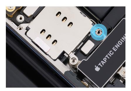
11. Tilt up the SIM reader and lift it out of the enclosure.
