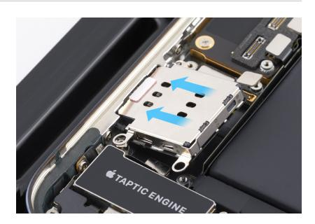
6. Use the black torque driver and Micro stix bit to install one new trilobe screw into the upper left corner of the SIM reader.
