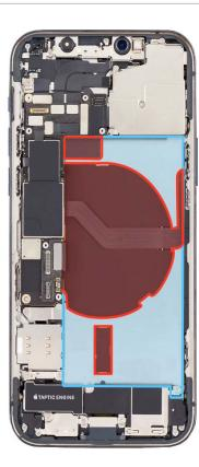
15. Insert the flat end of the black stick into one of the insertion points as shown. Ensure that the black stick is inserted into a point where the battery strip has been fully removed. Don't insert the black stick into a point where the battery tab or strip is broken.
