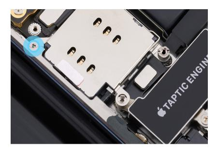
10. Use a torque driver and the super screw bit to remove the super screw from the lower right corner of the SIM reader. Set aside the screw.
