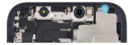
3. Use a torque driver and the Micro stix bit to remove the four trilobe screws from the camera cowling in the order shown. Set aside the screws.
