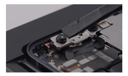
4. Align the replacement display adhesive over the enclosure with the top holes over the TrueDepth camera assembly and the bottom tab on the right.
