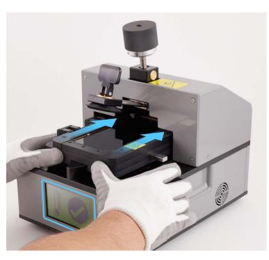
7. Turn the knob on the fixture clockwise to lower the suction cup as close to the iPhone as possible without touching the iPhone.
