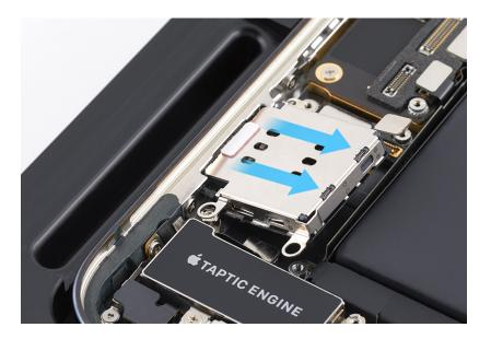
12. Use a torque driver and the super screw bit to remove the two super screws from the corners of the Taptic Engine. Set aside the screws.
