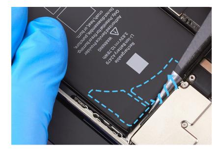
13. Repeat steps 11 and 12 to remove the remaining battery adhesive strip from the top of the battery. If you remove the entire adhesive strip, continue to step 14.
