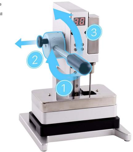
Wait until the timer on the display press beeps. Pull down the lever (1) and pull out the release knob (2). Then lift the lever (3).
