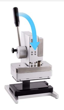
26. Wait until the timer on the display press beeps. Pull down the lever (1) and pull out the release knob (2). Then lift the lever (3).
