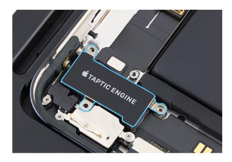
2. Press the end of the Taptic Engine flex cable to the connector.
