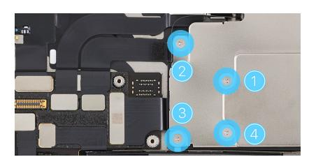
8. Use the gray torque driver and JCIS bit to install one new crosshead screw into the camera cowling.
