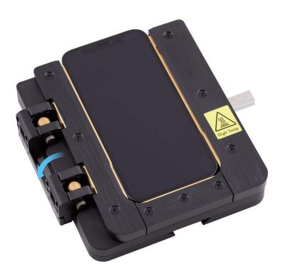
5. Put on the heat-resistant gloves. Align the cutout on the bottom of the pocket with the rail on the fixture. Slide the pocket with the iPhone onto the rail on the fixture.
