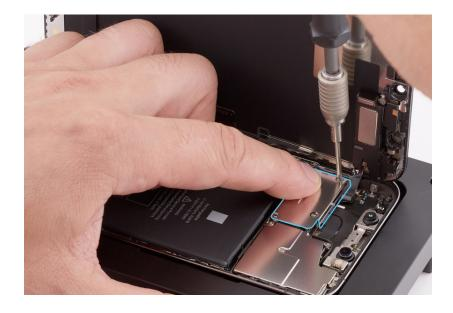
25. Use ESD-safe tweezers to remove the upper cowling. Save the cowling for reassembly.
