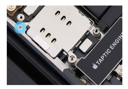
7. Use the gray torque driver and super screw bit to install one new super screw into the lower right corner of the SIM reader.
