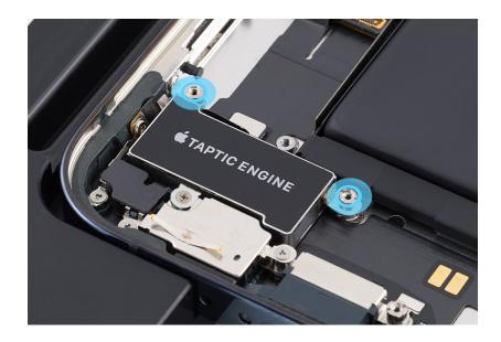
13. Use a torque driver and the JCIS bit to remove the crosshead screw from the bottom of the Taptic Engine. Set aside the screw.
