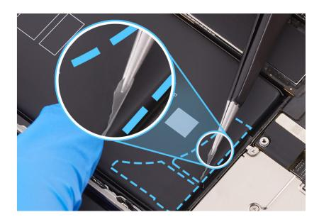
12. Keep the tweezers in the channel between the battery and the camera cowling. Continue to slowly twist the tweezers until you've removed the entire adhesive strip.
