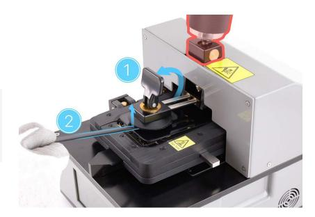
13. Press the eject button on the side of the pocket to release the pocket from the fixture.
