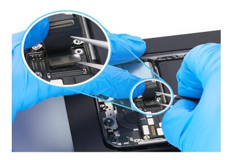
7. Gently hold the flex cables together and lift the cameras out of the enclosure.
